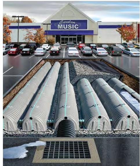
Water infiltrates through the surface and gravel substrate and is conveyed through the perforated pipe into a larger cistern, dry well, or other storage chamber.
