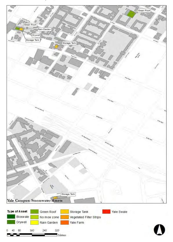
*Figure 5A: Approximate Locations of Yale University's Stormwater Assets (Central and Medical Campuses)*
