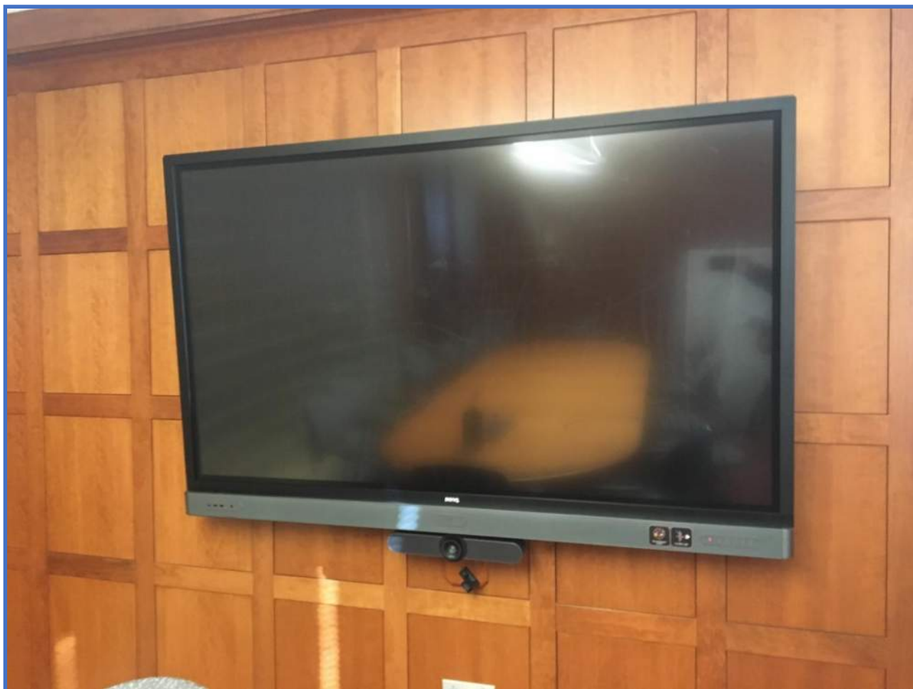
Conference Room Photo 5 – Wall Mounted Interactive Touch Flat Panel with UC Conferencing Wide Angle Camera/Beam Forming Microphone (Logitech Meetup)
