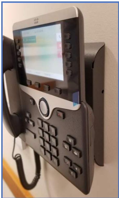
Telecom Outlet Photo 3 – Wall Mounted Cisco VoIP Telephone
