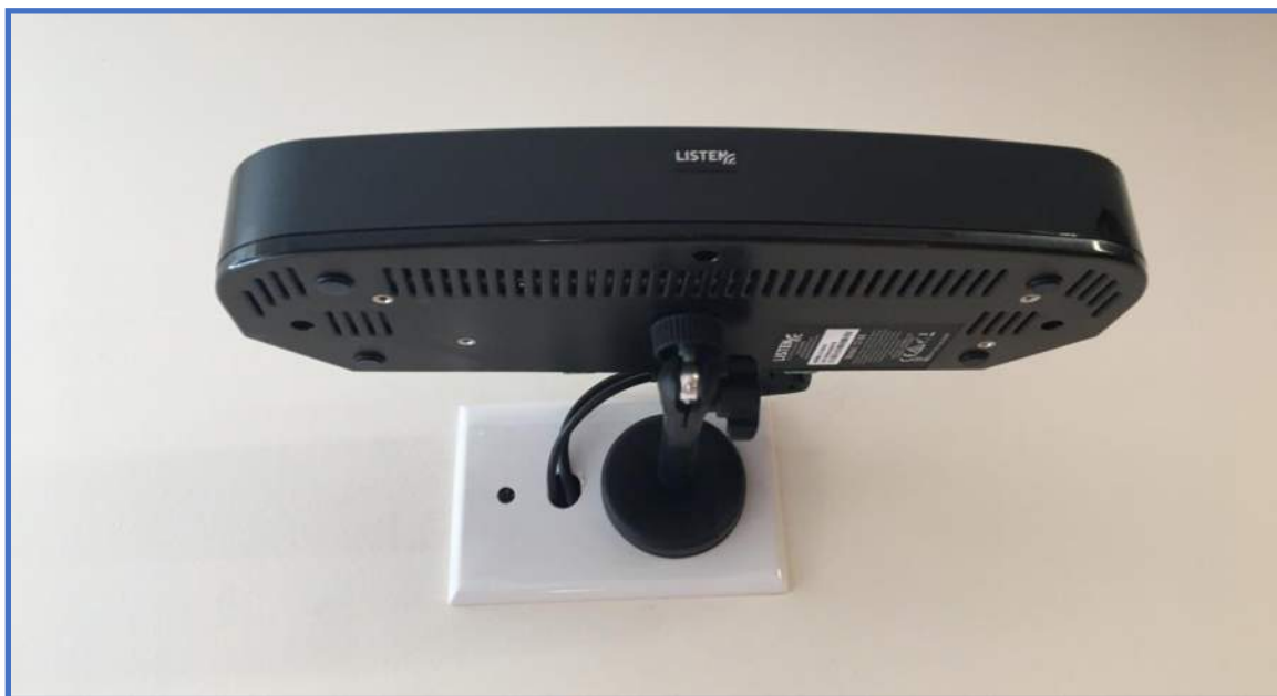
Assistive Listening System (ALS) Transmitter Photo 11 – Wall Mounted Infrared ALS Transmitter (Listen Technologies LT-84)
