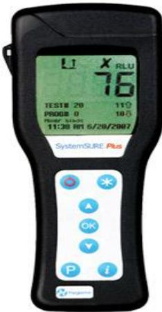
SystemSURE Plus is the next generation of the world's best-selling SystemSURE II ATP hygiene monitoring system. This new system uses state-of-the-art electronics with improved functionality, but still maintains its small hand-held design and affordability.
